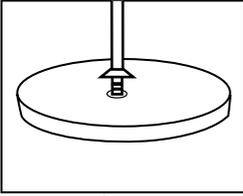
1. Insert pole into the hole in the base.
